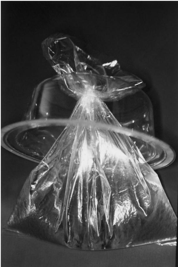
FIG. 2. The open edge of the pliable plastic bag is pulled through the hole of the container.
